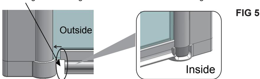
7. To change the handing of the stabilising bar **BSYS023**, unscrew where the arm attaches to the glass clamp and reverse. Place the stabilising bar onto the fixed panel. Mark the fixing point for the bracket to the wall. Use 6mm masonry bit, insert 1 wall plug **2SP12** and fix to wall with screw **2SY51**. Fasten the bracket to the glass keeping the washer on the outside of the glass. Attach cover caps to bracket. Fig 7.
