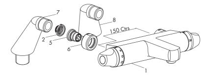
Note: The deck mounting legs are supplied complete with retaining nuts.
